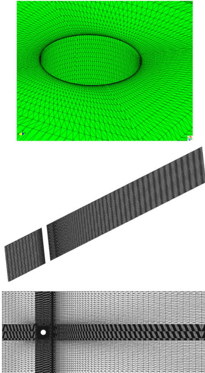
Figure 12. Flow past a cylinder. Details of the mesh used for the computations.
